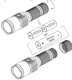
Note: After loading the batteries, the power indicator light will blink to indicate the battery voltage. Please refer to the "Power Tips" section of this manual for details.
